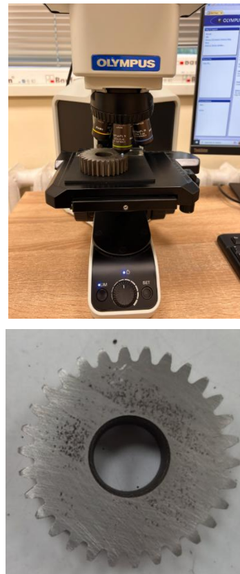
Fig. 1. Examination of a 3D-printed gear specimen using an Olympus microscope and gear sample.
