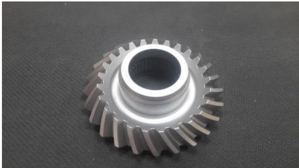
Fig. 7. Bevel gear with a circular tooth after processing (Photographer: S. Riabchenko).
