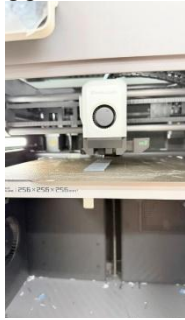
Fig. 3. 3D printing process of the specimen using the Bambu Lab X1E with AMS.
