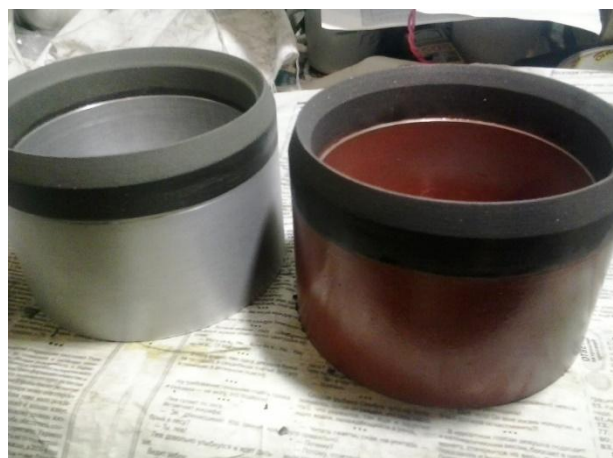
Fig. 6. Cup grinding wheels made of super-hard materials for processing a bevel circular tooth (Photographer: S. Riabchenko).
