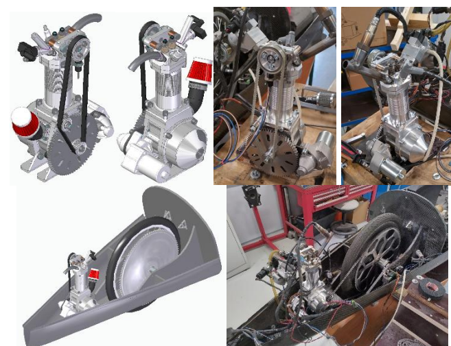
Fig. 12. Complete engine assembly in CAD (left) and after manufacturing (right).
