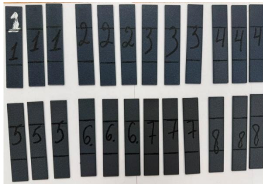
Fig. 5. Eight series of three 3D-printed carbon-filled composite specimens.
