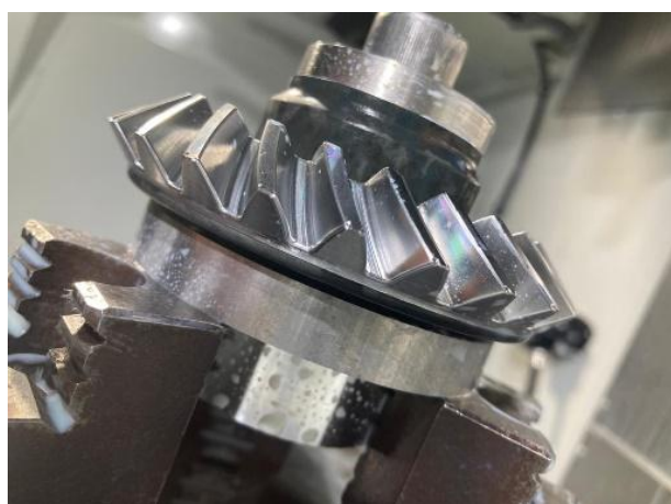
Fig. 4. Machining of the gear ring on a machine model "HAAS UMC 1000" (Photographer: S. Riabchenko).
