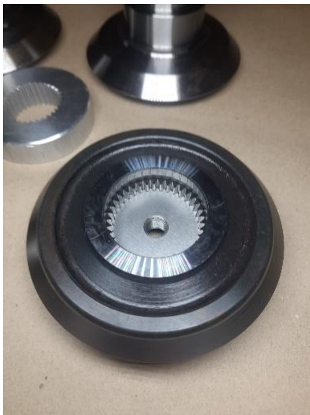
Fig. 3. Cut internal toothed splines and gauges (Photographer: S. Riabchenko).
